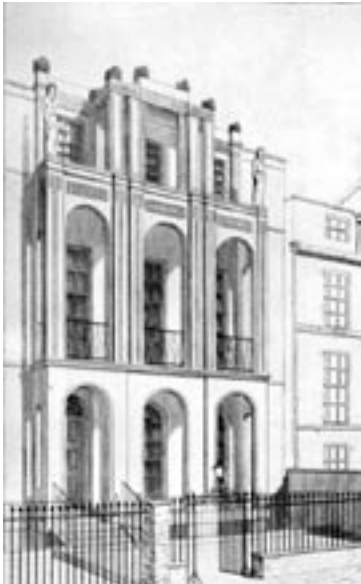
Soane's house, 1813-37, supports no entablature. Columns trophy their burdens directly, while arches web the wall.
